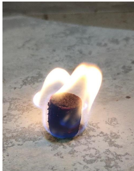
Record the start time of burning using a stopwatch, wait until the bio-coke briquettes are completely burned, and record the last time they burn.
