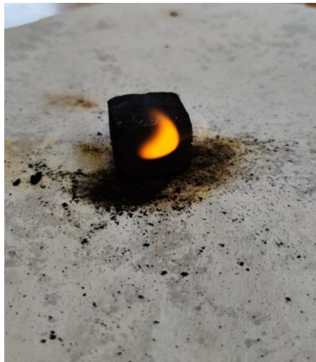
Prepare the control and perform a combustion test with the same treatment burned and record the duration of the last flame burning.
