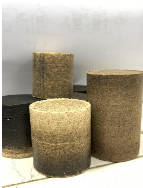
Stored in a desiccator to keep the bio-coke from getting damp.
