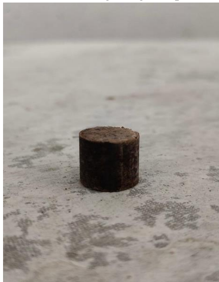
Prepare 12 mm briquettes at a temperature of 170°C, make sure the test room is free from wind and there is not much interference.
