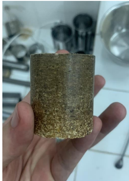
Bio-coke briquettes from the utilization of agricultural waste from corn cobs
