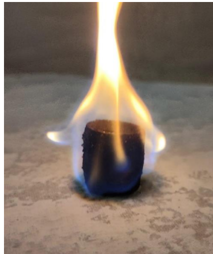
Record the start time of burning using a stopwatch, wait until the bio-coke briquettes are completely burned, and record the last time they burn.
