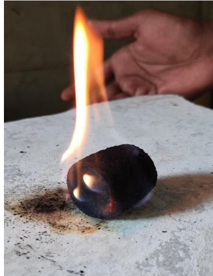
Also, the 30 mm size bio-coke briquettes were burned and the burning time of the last flame was recorded.
