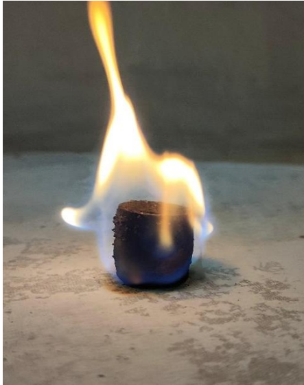
Carry out the same treatment on a 20 mm size burnt and note the length of time the last flame burns
